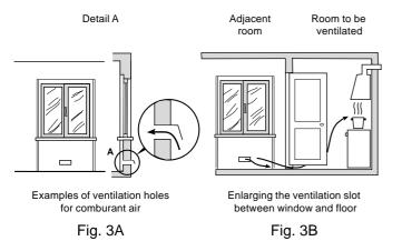
The air inflow may also be obtained from an adjoining room, provided the latter is not a bedroom or a room where there is a risk of fire, such as garages, mews, fuel stores, etc. and is ventilated in compliance with the standards in force.
